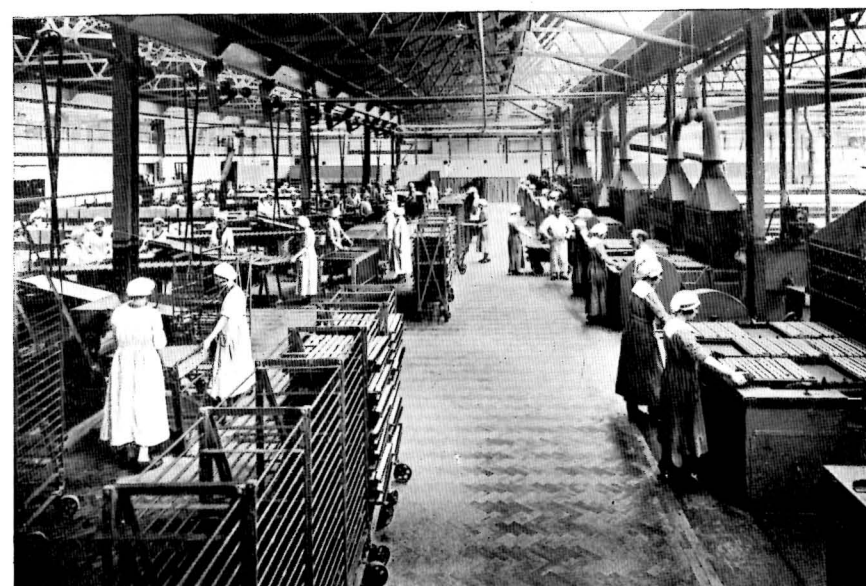
After their 50-foot journey through the Gas Heated Ovens the Pans are being taken off and placed on Racks to cool
