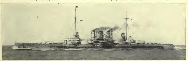
The Dreadnought Thuringen, one of the Helgoland type, a class completed in 1911 and 1912, having a displacement of 21,000 tone, a speed of 22 knote, and carrying twelve 12-in., fourteen 6 in. guns, fourteen 24-pounders, and six 20 in. torpedo tubes.
