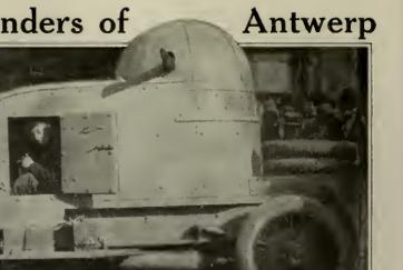
A Beigian armoured motor-car that has made sortles from Antwerp and put marauding Germans to flight. The driver is well protected, and at the back of the car is a revolving turnet which permits a machine-gun to fire in any direction.
