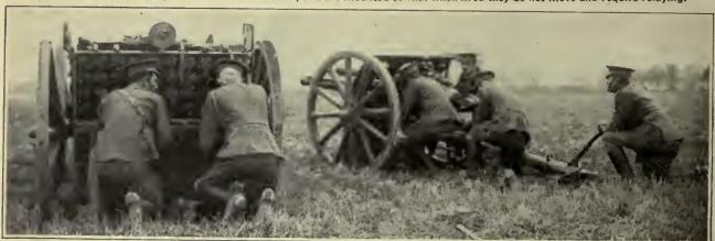
A British field piecs in action, showing its caisson or ammunition waggon. Field guns are fitted with shields to protect the men working them against builets from the enemy's rifles and shrapnel fire. The range of the guns varies from 5,500 yards to 9,000 yards.
