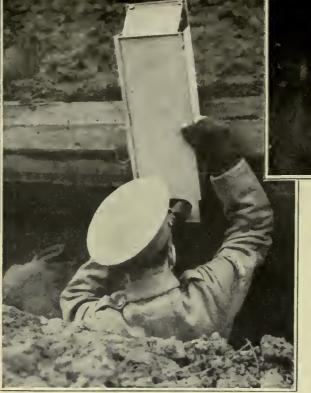
Soldier manipulating a new military periscope. This invention was used extensively at the front, and proved very serviceable as means of watching the enemy's positions from within the trenches.
