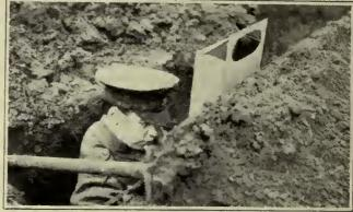
Another photograph ehowing how a British eoldier, safely hidden in the trenches, was able to observe the movements of an enemy, which are reflected by means of glasses in the periscope.
