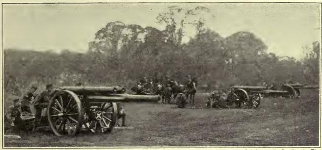
Soms 60-pounder guns which proved of remarkable accuracy of aim and rapidity of firs in the hard fighting on the Continent. The two cylinders surmounting the barrel are technically known as "recoil chambers," and absorb the terrific concussion caused by the explosion of the charge. Without these the weapon might perform a somersault in the air and fall many yards in the rear of its position.
