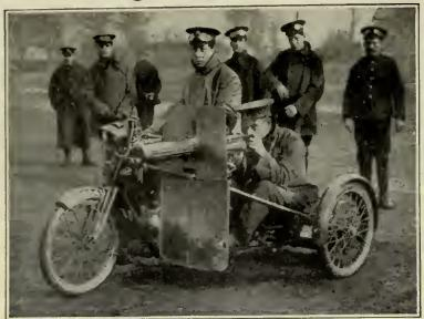
Corporal Frank Cody, son of the late Colonel Cody, in charge of a field artillery motor-cycle. The gunner is alming the machine-gun from behind the bullet-proof shield with which the machine is fitted.
