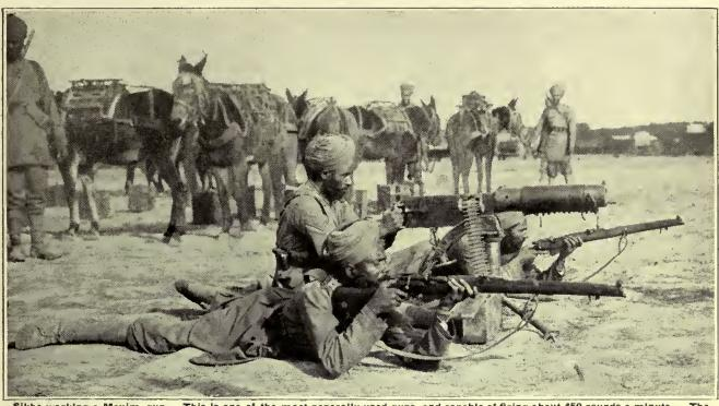
Sikhe working a Maxim gun. This is one of the moet generally used guns, and cspable of firing about 450 rounds a minute. The belt of cartridges is seen passing through the feed-block while the gunner directs the fire by mesne of two handles at the rear.
