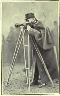
French officer using the telemeter, an instrument for calculating distances.
