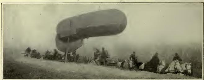
gasbag is transported, attached to a waggon carrying the inflating apparatus. The curious open, tail-like appendix acts as a sort of rudder, and holds the balloon stsady when aloft by filling with air according to the force of the wind.
