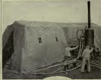
Coliapsible field steam laundry used in the German Army. The structure could be taken to pieces easily and conveyed to another part of the front. Right: Bathing-waggon being worked outside a tent containing baths of hot water.
