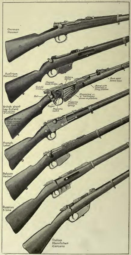
The rifles used by the belligerents, showing in detail the working of the British Lee-Enfield. This, the latest British Government pattern, known as "Mark III.," and the result of a series of improvements on the 1887 pattern, has a magazine holding two "chargers," each containing five rounds, so that the magazine is filled with ten rounds in two motions. Unlike the German Mauser, our rifle is fitted with a cut-off, which enables it to be used as a single-loader. The barrel is 25 in. long.
