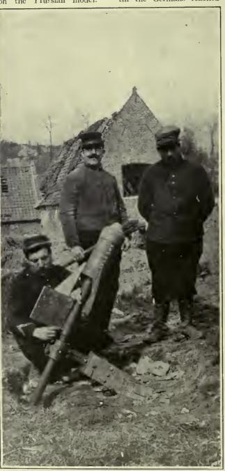
French soldiers fixing an serial torpedo to be fired against hostile sircrsft. Note the wings, which assist in the projectile's flight.
