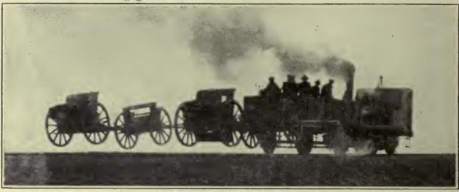
Field-guns leaping over a seriee of travsrse ralis, while being towsd by a locomotive. This was one of the eevere teets to which new German guns were subjected at the great Krupp Works in order to make certain that their carriagss can withetand heavy shocks.
