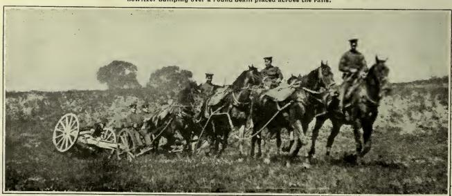
Teeting a new field-gun for horse artiliery over rough ground near the Krupp Works at Eeeen. These severe trials were made to test the power of the guns' mechanism to withstand ehocks while in motion without becoming deranged.
