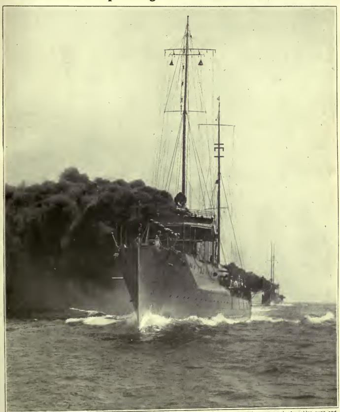
Remarkable photograph of the Parker and the Benham, two of America's ewifteet deetroyers, steaming et fuil epeed on a epecial run. They are eleter ships of the Alwyn class, completed in 1914, and are of 1,010 tone displacement and 16,000 h.p., with a designed epeed of 29 knote. They carry a complement of 98 officers and men, and their
