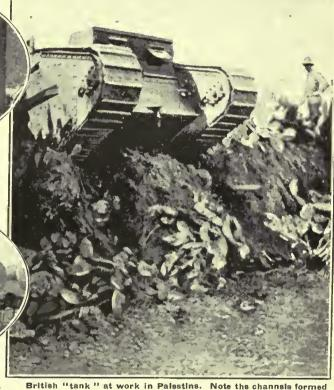
in the bank it has surmounted by means of its caterpillar wheels.
