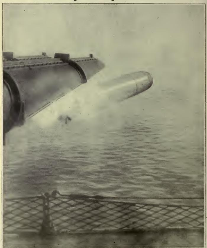
Torpsdo practice aboard the U.S. destroyer O'Brien. The O'Brien is one of six destroyere of the Cushing class, laid down in 1913. Her displacement is 1,052 tons, and her designed speed 29 knots. Armament: Four 4 in., 50 cat., guns, and eight 18 in. torpedo-tubes (twine). Complement: 98 officers and men. While prepared to
